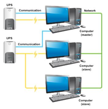
You can even have a UPS that has the serial port connected to a system that it's not feeding. Sometimes a PC will be close to a UPS that needs to be monitored, so it's drafted to supply a serial port for the purpose. This PC may in fact be getting power from some other UPS. This is not a problem.
