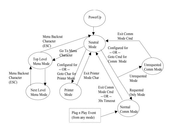
The following diagram illustrates the states for Baud Rate, including the means of transition.
