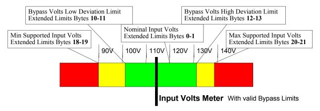
Otherwise (On-Line UPS, no Bypass Meters or Bypass Deviations not valid), draw the Input Meter like this:
