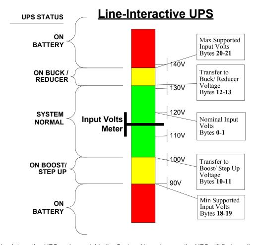
For Line-Interactive UPSs, when outside the System Normal range, the UPS will first use the Buck / Boost feature to try to restore the output to within regulation without going On Battery. However, if the utility voltage falls outside the Buck / Boost limits, then the UPS will transfer to On Battery.
