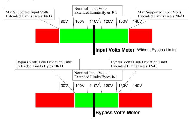
Else (On-Line UPS, but no Bypass Meters), if the following relationships (all Extended Limits data) are true: Nominal Input < Bypass Volts High Deviation (bytes 12-13) < Max Supported Input Volts (bytes 20-21) AND
