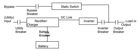
Bypass: in the Meter Map, refers to measurements for a physically separate utility feed than the Rectifier Input. UPSs with a single utility feed (where Bypass and Rectifier Input are always tied together) should report Input (not Bypass) Voltage and Frequency. Some current models violate this convention and report "Bypass" meter values, so communication software must accommodate this deviation.
