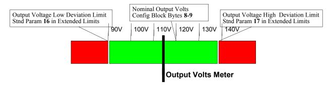
If the Min/Max limits are not provided in the Table of Standard and Custom Parameters in the Extended Limits block, then just show it as a digital readout.
