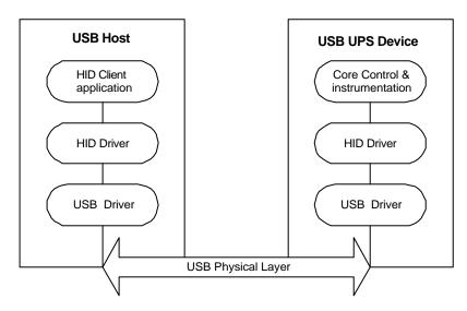
Figure 1: General diagram of communication layers between USB host and device using HID.
