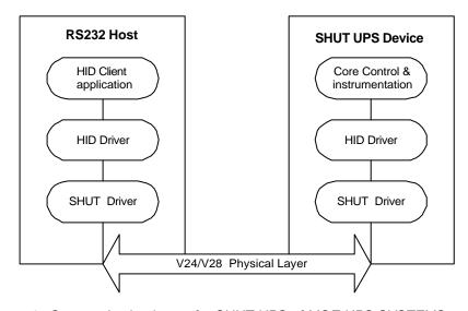
Figure 2: Communication layers for SHUT UPS of MGE UPS SYSTEMS
