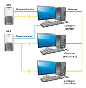
You can even have a UPS that has the serial port connected to a system that it's not feeding. Sometimes a PC will be close to a UPS that needs to be monitored, so it's drafted to supply a serial port for the purpose. This PC may in fact be getting its own power from some other UPS. This is not a problem for the set-up.
